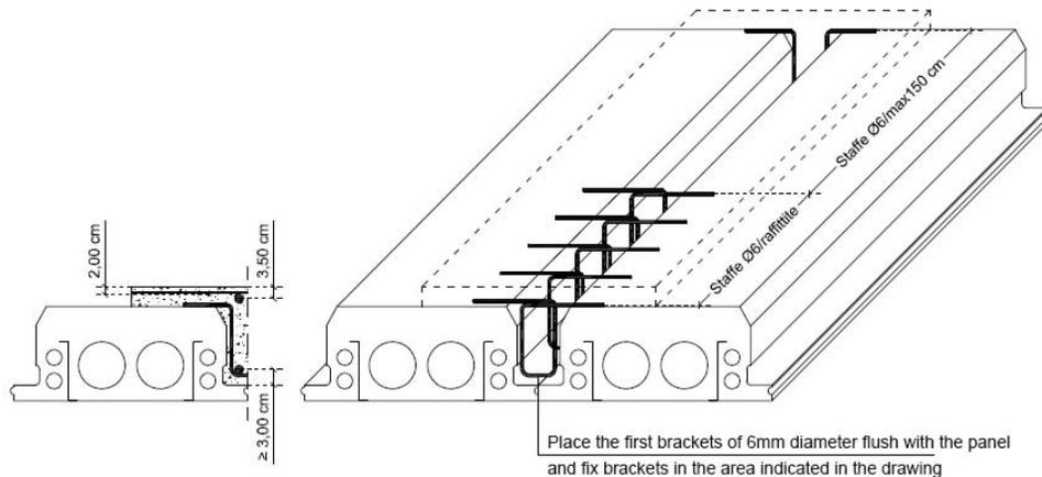
Place the first brackets of 6mm diameter flush with the panel and fix brackets in the area indicated in the drawing
